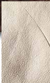
Scratches Smooth to the touch, these rub marks may accept dye with slight variation to the surrounding area.
